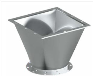
adapter sleeve (circle - square) D = 150—300 square = 200x200 250x250 300x300
